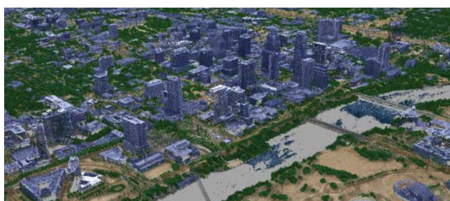
Merged Classified Lidar Point Cloud and Intensity Returns
